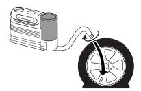
Note: When the sealing compound is first added into the tire, the air pressure gauge reading on the compressor unit may indicate a higher value; this is normal and should be no reason for concern. The pressure will drop after about 30 seconds of operation. The 344
